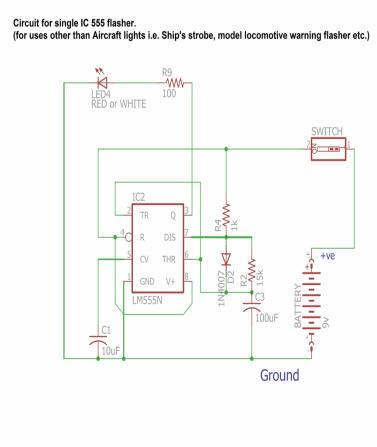
Navigation lights for model aircaft (9v) (example as single circuit)
