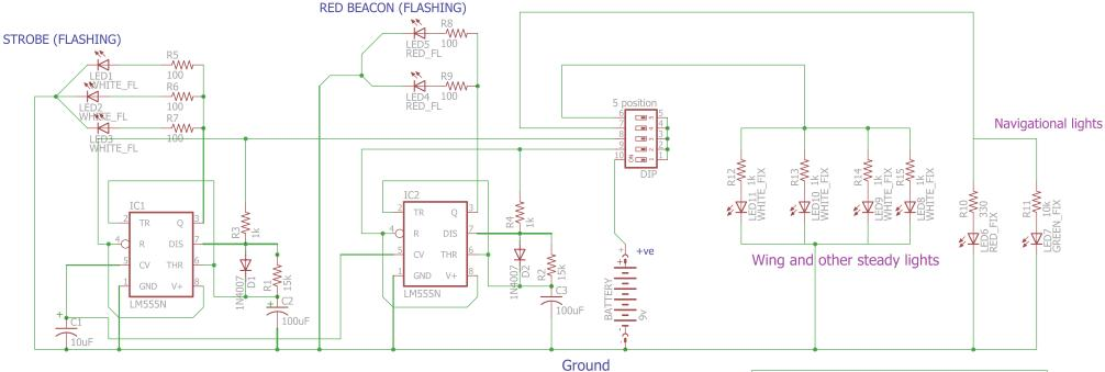
Navigation lights for model aircaft (9v) (5 position DIP switch for individual control)
