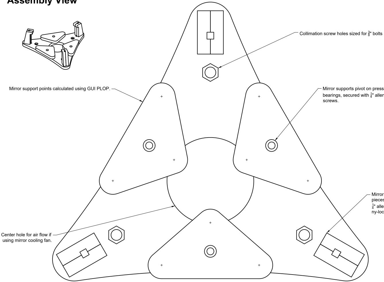
Mirror supports pivot on press-fit spherical bearings, secured with  $\frac{1}{4}$ " allen head cap
