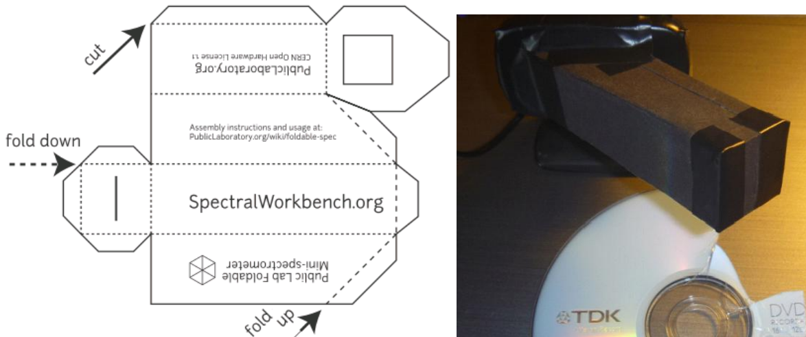
Fig. 2. Foldable paper spectrometer construction after downloaded plans from https://publiclab.org/sites/default/files/8.5x11mini-spec3.8.pdf
