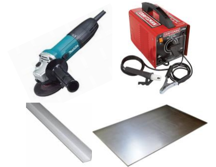
Angle grinder, manual arc welder, galvanized angle profile and galvanized steel sheet (5mm)
