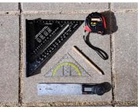
A: PencilB: Protractor triangleC: RulerD: Measuring tapeE: Rafter Square
