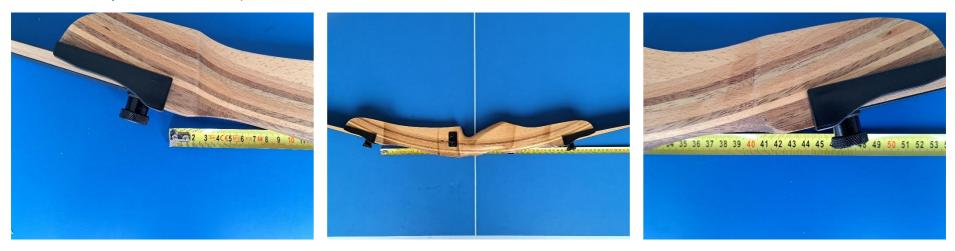
As shown in the photo's the distance between the points on which the handle will rest are 44 cm apart.
