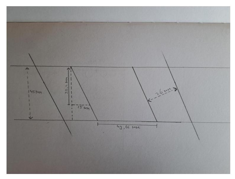
F: Sketch of the position of the dowels in the lower joint
