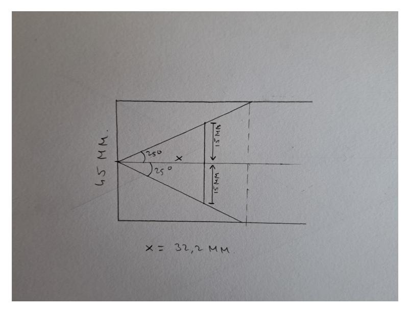
H: Measurements to determine the 25° angle
