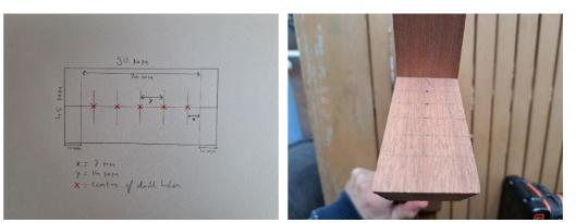
On the top of Beam 5 the space between Beam 2/3 & Beam 4 was measured. This was approximately 90 mm. From both ends 10 mm was left alone and the other 7 cm was used to space out the holes for the arrow tips. Draw a centre line on the top side of Beam 5 and measure out the 70 mm with the 10 mm spare on both sides. Use this for the next dimensions.
