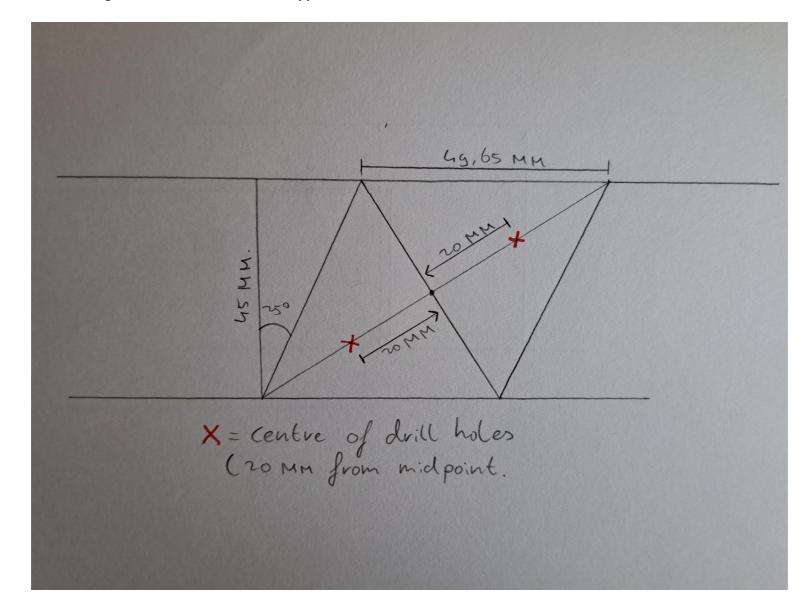
I: Measurement for drawing out the dowel holes for the support blocks
