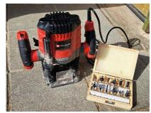
Q: Router drill with drill bits
