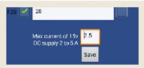
Enter 2.5 in this box and press 'Save' The App will now limit the output current to 2.5 amps. If you are using a 2 amp DC power supply, enter 2.0 into this box and press 'Save'. The App will limit the output to 2 amps.
