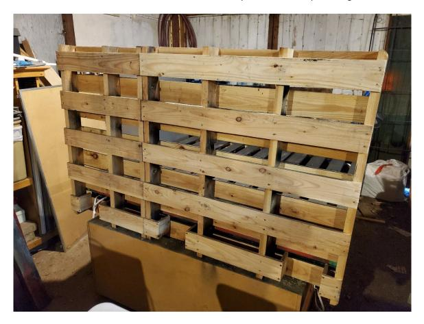
I made simple cuts at the bottom edge to make room to drill a hole and connect the bottom level to the headboard. I did the same for the headboard to the top level.
