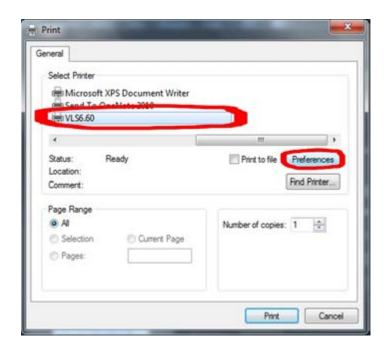
13. Set the colors according to your desired vector cuts or rastered objects. Set settings for colors in this window before moving to UCP. If not, the colors will not have the option to be changed from vector to raster or vice versa, leaving the only option available as skip.
