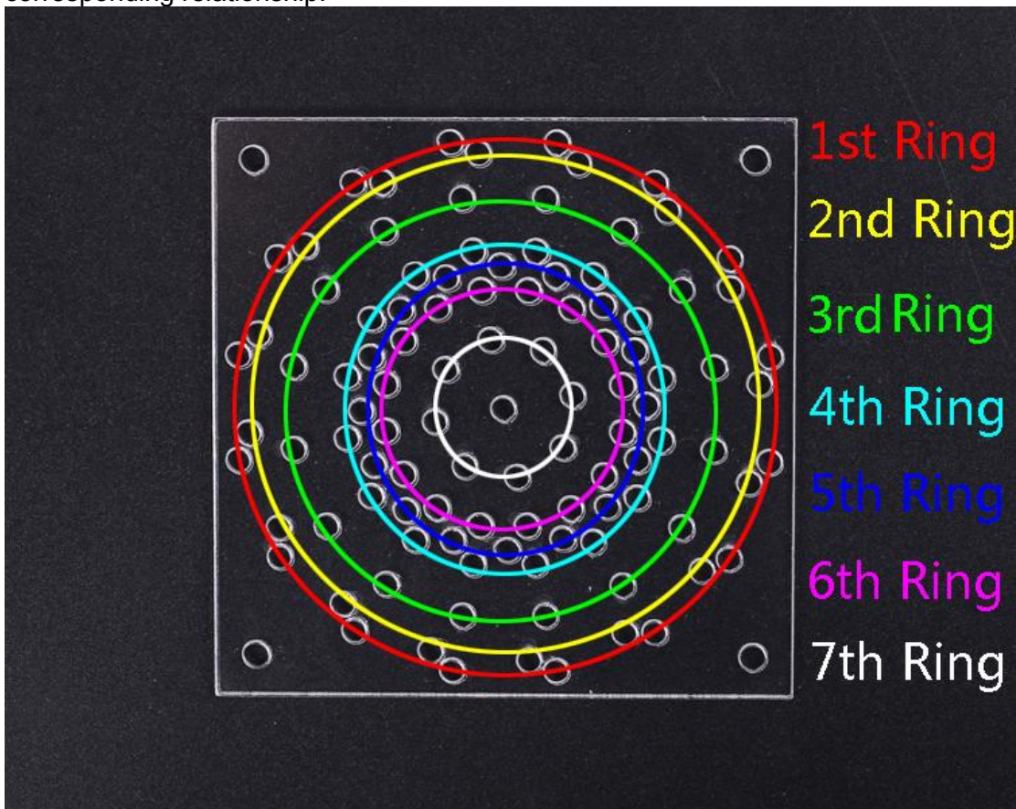
Step 8: Acrylic Welding Template Ring,LED Layer and Anode solder pad corresponding relationship.
