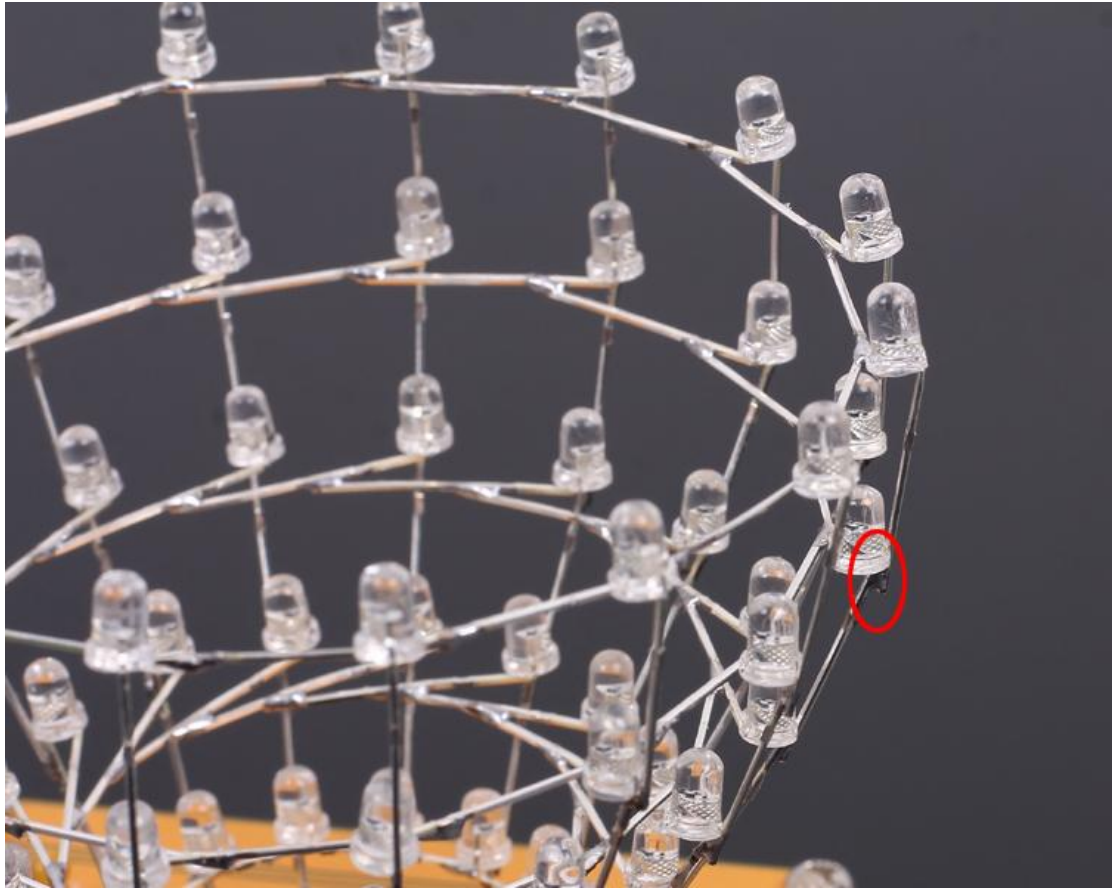
Step 14: Install 6th~8th layer, but bend the LED pins in different ways.
