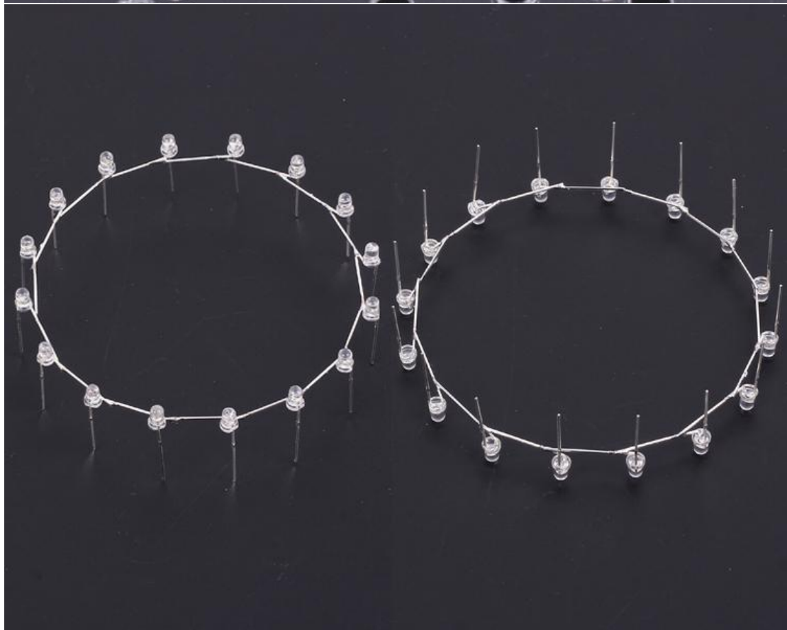
Step 11: Install the 2nd Ring to the 6th Ring total 8pcs LED rings as Step 10. NOTE: It is need to install 2pcs the 2nd Ring and 2pcs 2pcs 3rd Ring.Others
