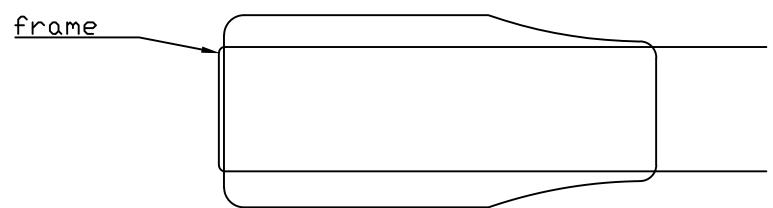
FRAME STEP 2: CUT THE ENDS OF THE FRAME 4" PAST THE FRAME SHEET, FILE SMOOTH AND ROUND. BEND THE TIPS OF THE BOTTOM OF FRAME AT I" FROM THE END. BEND ROD AT FRAMESHEET AND TUCK ENDS INTO CORRUGATION.
