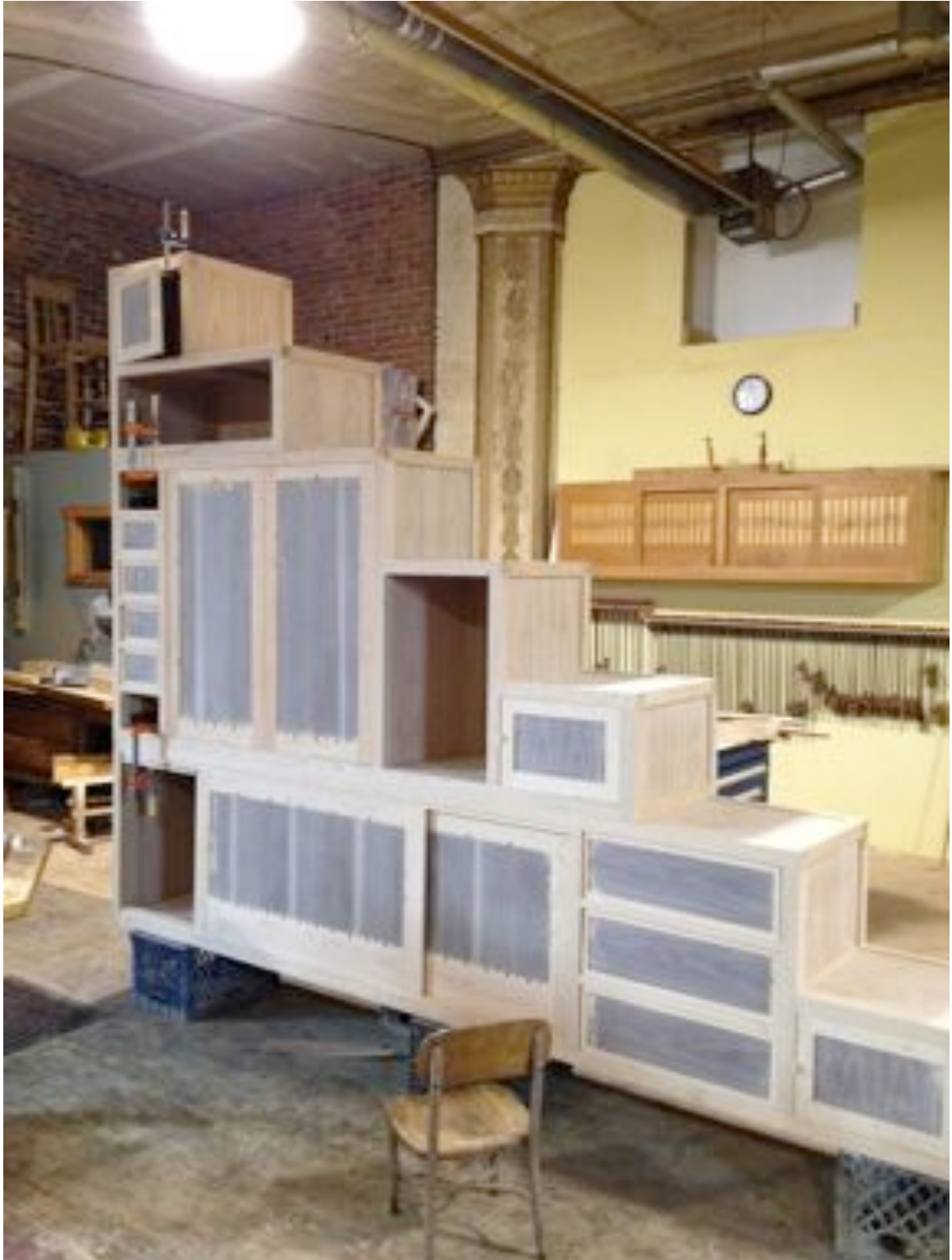
38. On to the sliders; I installed the decorative latticework of the sliders. My first step was to size all the sticks, disregarding the need for joinery.
