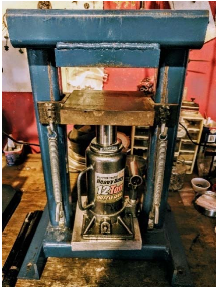
Figure 3: A 12-Ton press frame based on a very similar design to this one
