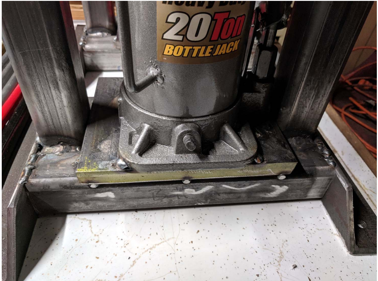
Figure 13: Steel base plate with angle iron legs
