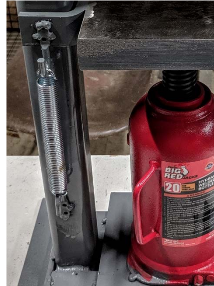
Figure 20: C-277 welded - only slight tension at rest
