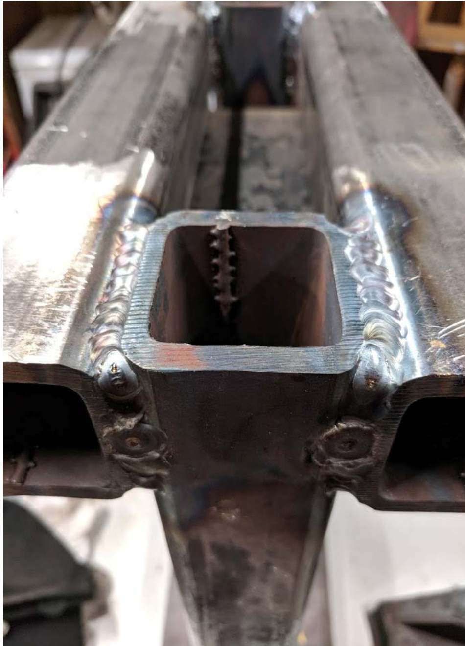
Figure 9: TIG Wlded Stress/Pressure Frame
