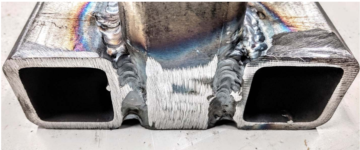
Figure 12: Sanding frame to sit flat and flush with table and angle iron
