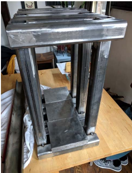
Figure 8: Tack Welded Frames
