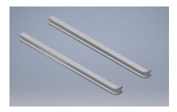
**Step 3:** Place the two top plates on the runners so the holes line up with those on the runners and put the one with two hole on the front near the curved ends of the runners.
