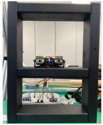
4. Once the location is finalized, take 2 self-tapping wood screws and drill through the main base of the eye mechanism at arbitrary locations to ensure strong fixation of the eye mechanism to the supporting structure.
