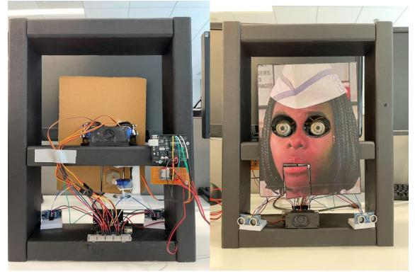
At this point your assembly has been completed and will properly function pending power being provided to each Arduino. We decided to power the device using 9V wall plugs into the associated Arduino ports. Enjoy your animatronic face of Ed from Good Burger!
