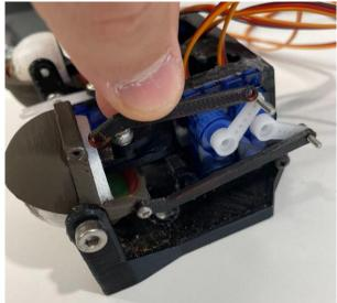
12. Attach the eyelids to the main base but do not connect any servo arms to the eyelids at this point. Make sure the eyelids are free to rotate in the housing without significant friction.
