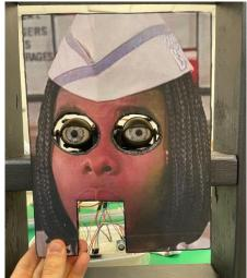
3. Place the eye mechanism on the middle shelf of the supporting structure and align it with the face in a location that lines up with the eye cutouts of the face. (Note: Be sure to offset the location of the eye mechanism behind the face to ensure the servo arm or eyelids contact the back of the face cardboard.)
