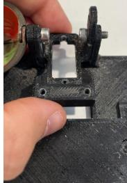
2. Insert the servo into the sub-base and fix it into place with 4 or 6 mm M2 screws. This servo will be in charge of side-to-side or x-axis motion.
