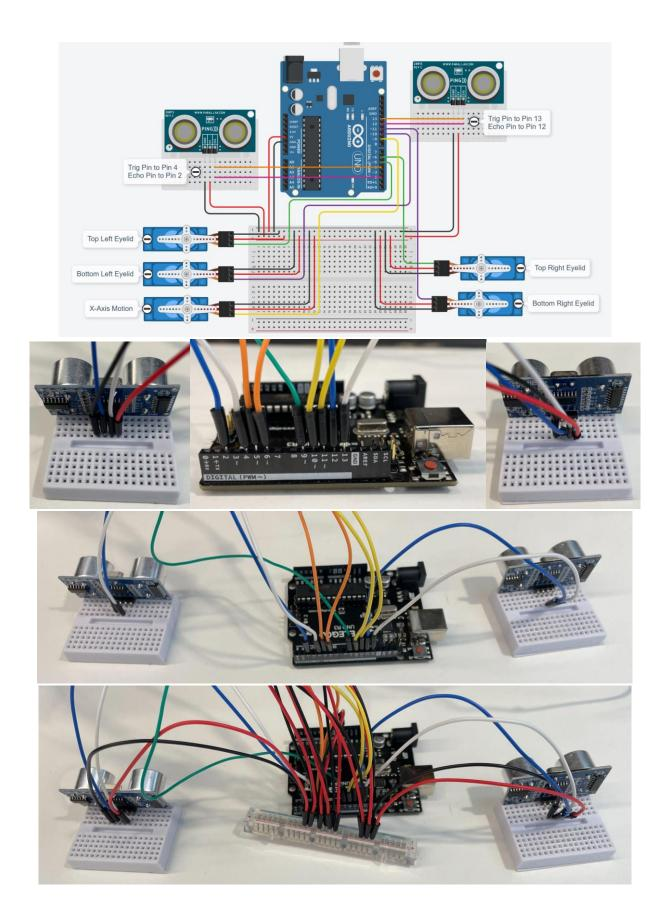
Once all components are wired, this is the opportunity to link all the servo arms to their respective servos. To do this, ensure the eyes are facing forward and in a neutral position. For the eyelids, ensure they are closed and centered along the eye diameter. After this is verified, attach the servo arms to their respective servos.
