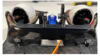
9. Attach 4 servos to the servo block using the self-tapping screws given with the servos. The correct orientation of these servos are shown in the below picture.
