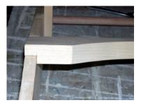
**9** - After cutting out part M, you need to rabbet the ends so the part fits flush to the top of parts  $\bf A$ . Cut out a 1/2" deep x 3/4" wide (1.25cm x 1.9cm) rabbet in the underside being sure that it also fits easily into place between the side panels  $\bf A$ .
