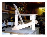
14. The chair is now assembled, and ready for finishing. If your are plugging the screw holes, I recommend a tapered plug cutter, like the Veritas Cutter from Lee Valley Tools or the hex shank tapered cutter from Rockler. Glue the plugs in place with exterior waterproof glue, let dry, then cut off the excess with a chisel or Japanese saw. The rest can be sanded smooth with a random orbital sander. Touch up the plugs with primer, if painting the chair.
