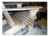
13 - Rip all seat slats **S** to the size shown on the parts list. Attach all seat slats with one 1 5/8" (4.2cm) # 6 screw in each side being sure to drill pilot holes into the side panels **A**. Use the templates as spacers to evenly space the seat slats between the front and back slats parts **C** and **R**.
