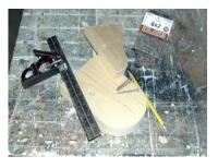
**4** - Mark the center lines on parts **H**, being sure that the pivot holes are in the correct location, since parts **H&I** are opposite under each arm. Be sure that the pivot holes are closer to the back of the chair and line up with the upper holes in parts **D. GLUE** and screw part **I** in place with three 2" (5.1cm) screws, being sure to drill pilot holes first.
