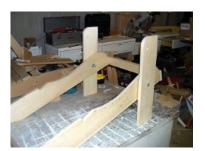
**3** - Add a flat washer, then a lock washer and tighten the nut. Assemble the second leg to form the carcas seen at the left. Be sure the bottoms of the side panels **A**, rest flat at the back.
