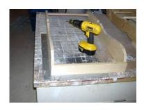
**1** -Begin assembly by cutting the dowel part **B** to length and screwing in place between parts **A**, the side panels, with 2" (5.1cm) screws. Next attach the front slat **C**, with two 1/58" (4.2cm) screws on each side, to the front edges of parts **A**, flush with the bottom edge, or with a 1/4" overlap as I prefer. This will give you a carcass to work with. Check for square by measuring corner to corner, both ways. If the carcass is not square, the chair will not fold.
