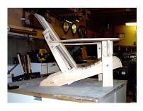
**15 -** To recline the back, sit in the chair, reach your arms back around the back slats, grab the back supports **E**, and pull forward. To put it back in the upright postion, reverse the process. Check to be sure there is no binding at part **R**. The supports **E**, should fold against the back of part **M**. The front legs may tilt back slightly when you lean back. If you don't want the chair to recline without getting out of the chair, add another dowel in front of dowel
