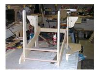
**6** - Assemble the back supports parts **E** with the dowel **F**, cut to length. Screw the dowel in place with 2" (5.1cm) screws, being sure the back supports are square to each other. Place the assembled section in front of the rear dowel part **B**, being sure that the straight perpendicular front of the assembly, is facing the front of the chair.
