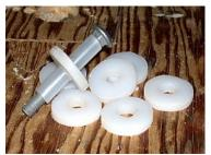
**8** - Here you can see the final assembly of the bolt, plastic waterline and plastic washer ready for asembly.
