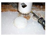
**6** - Using the UHCW plastic, make 8 washers using the 5/8" (16mm) hole saw. The Lee Valley plastic is already 1/4" (6.5mm), but if you buy 3/8" (9.5mm) plastic jig stock at Rockler, rip or plane it to size. Use a cutting blade to trim off the plastic burrs to make the washer smooth.
