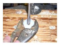
**7** - Using a woodturners center finder, mark the centres of all washers and drill the 1/2" (13mm) holes, holding the washers with vise grips, flush to the drill press table. Trim off the burrs so they run smooth against the wood surfaces.
