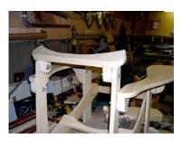
**8** - Assemble the back support pivot parts **K** in the upper holes on the inside of back supports **E**. Be sure that the tops are angled towards the back of the chair. Center the back support part **L** on the pivots, drill pilot holes, **glue** and screw in place with two 2" (5.1cm) screws into each pivot.
