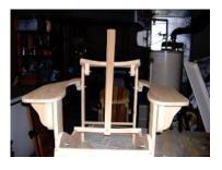
**10** - The back pieces can now be assembled, starting with the middle slat  $\mathbf{N}$ , centered at the top on part  $\mathbf{L}$ , and at the bottom, in the curve on part  $\mathbf{M}$ . Overhang 5/8" (1.6cm) below the bottom of support  $\mathbf{M}$ . Use one 1 5/8" (4.2cm) screw at the top and bottom of each slat, being sure not to set the screws too deep.
