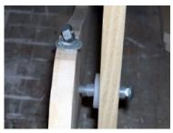
**2** - Next, bolt on the front legs **D**, on the **OUTSIDE** of parts **A**. Cut a piece of tubing to 1 5/8" (4.15cm) and slide it over the bolt to the square head under the crown. Push the bolt through the lower hole of part **D** being sure that the curve at the top faces the back of the chair. Add the plastic washer, then push the bolt through the front hole of part **A**. Double check the length of the tubing to be sure it doesn't protrude past the inside of part **A**.
