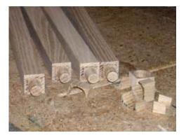
3 - Mark all mortise positions on parts A & B. Using the drill press and a 1/4"(6.35mm) brad point bit, cut through mortises and trim the insides square with a sharp chisel. The mortises in parts B are closer together than parts A, so when the cross braces are added, they will fit inside each other.
