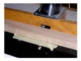
8. Mark each leg as shown, for the dados to accept the doweled ends of the cross bars. Set up the router table with a 9/16" (1.4cm) straight bit, set 3/8" (1cm) from the fence. Mark a piece of masking tape on the table surface as shown, with the start and stop edges of the bit, and line up the work pieces with the start and stop lines marked on the wood. You will need to make 2 passes in oak or any hardwood, to get to the 5/8" (1.6cm) depth.
