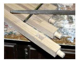
4 - Mark the ends of parts C, the cross braces, for the tenons that fit into the mortises in A & B. Cut the tenons at the radial or table saw, & dry fit in the mortises.
