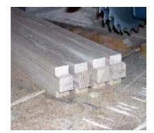
7.Mark 2 legs as D, and 2 as E. The dados you will be cutting are opposite on D & E, but the leg turns around and is at the opposite corner.....ie:D is one front and one rear opposite back leg.
