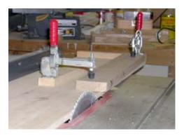
15. Place the arms flat on the work surface, tapered sides out. Clamp the completed leg assembly together with a 1/8" (3mm) spacer between the legs, upside down on the arms as shown. This is easier to mark the mortise locations on the arms, than measuring. Make sure the leg assembly is centered and to the edge of the 3 1/8" (8.25cm) line, and mark the edges of the tenons to give you the mortise locations.
