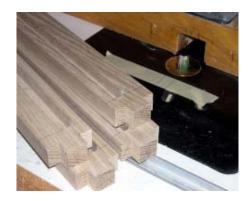
9. Mark each leg with cross hairs for the 1/2" x 5/8" (1.2cm x 1.6cm) deep holes at the bottom of each leg, being sure that they are on the same side as the slot above. Follow the diagram for correct positioning, 2" (5.0cm) from the bottom & 3/8" (1cm) from the inside edge as the dado above. Set up the drill press with a 1/2" (1.2cm) Forstner or brad point bit, drilling a 5/8" (1.6cm) deep hole. File the dowel ends to give smooth movement in the holes.
