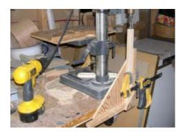
NOTE:You can substitute the dowel cutter process, by drilling 1/2" (1.27cm) holes into the ends of parts A & B, and gluing in 1/2" (1.27cm) hardwood dowels. If this is done, the parts will have to be trimmed by 1 1/4" (3.2cm), so the dowels will protrude out 5/8" (1.6cm) on each end, making the parts 15" (38.1cm) long.
