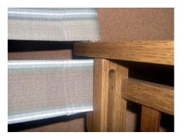
23. With the material completed, lay the folded, stained and finished chair on the work surface, with a board between the upper cross braces as shown. Staple the seat flush to the lower edges of the cross braces, then nail on the brass upholstery strip over the staples. The material should be tight when the chair is completley open. It will stretch somewhat as you use it.
