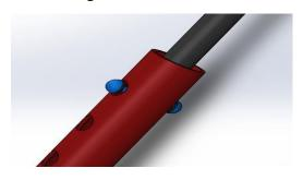
To adjust the retraction length of steering column the button is pressed and the sliding rod easily slides down and can be adjusted. This gives more space for the driver to get off/get in easily.
