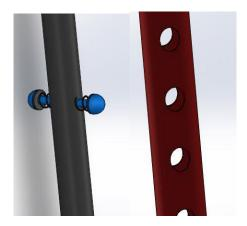
The outer rod has holes to allow the buttons out and lock in sliding motion. It also locks the rotating motion.
