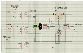
In the above circuit the throttel is replaced by a singel cell for simplicity. A 2 pole 6V relay and a 1 pole 6V relay is used for switching purpose as shown above. A voltage rgulator is used to regulate the voltage to the controller.
