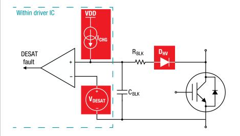
Figure 44: Typical DESAT circuit implementation
