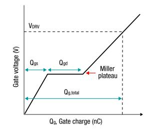
*Figure 7: Power device gate charge plot*
