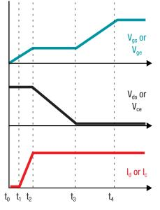
Figure 42: Power switch turn-on waveforms
