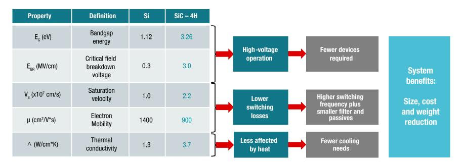
Table 1: Power device material characteristics
