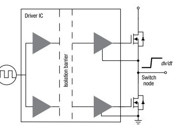
Figure 28: Isolated dual-channel driver
