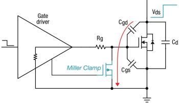
Figure 33: Gate driver without Miller clamp
