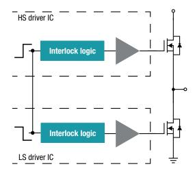
Figure 25: Two single-channel drivers with interlock
