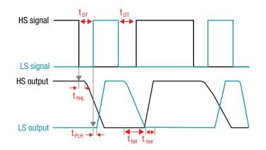
Figure 18: Propagation delay effects on dead time
