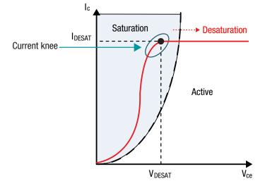
Figure 41: I-V curve of an IGBT
