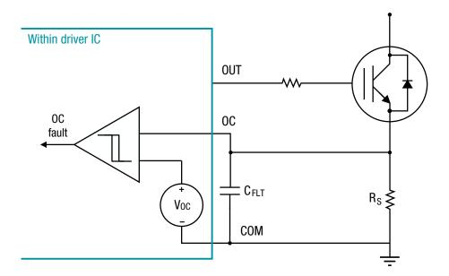
Figure 46: Overcurrent using a FET with integrated current scaling
