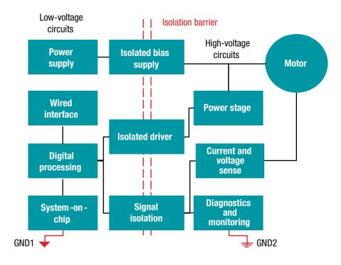
Table 5: Traction inverter block diagram
