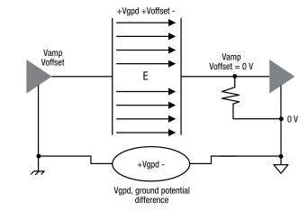
Figure 4: Capacitive isolation
