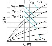
Figure 19: IGBT and SiC MOSFET I-V curves
