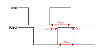
Figure 13: Pulse-width distortion
