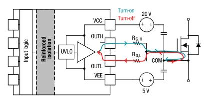
Figure 9: Driver with split outputs
