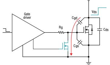
Figure 35: Gate driver with internal Miller clamp
