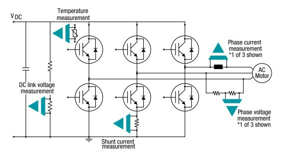
Figure 29: Isolated sensing in a three-phase motor-drive system
