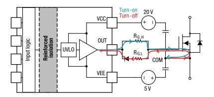
Figure 8: Driver with a single output
