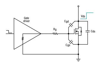
Figure 6: Power device input capacitance
