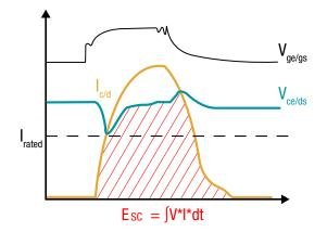
Figure 39: Power loss during a short circuit
