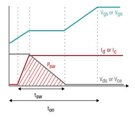
*Figure 10: Device turn-on switching losses*
