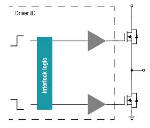
*Figure 24: Dual-channel driver with interlock*
