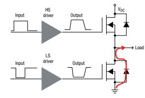
Figure 12: Synchronously switched half bridge
