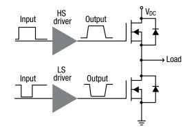
Figure 17: Hard-switched half-bridge configuration
