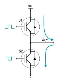
Figure 23: Hard-switched half bridge
