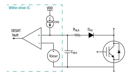
Figure 43: Typical DESAT circuit implementation
