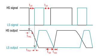
Figure 14: Effects of propagation delay mismatch
