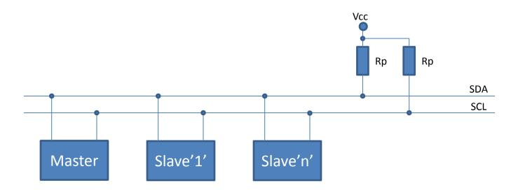
The output stage of the SDA and SCL lines are know as Open Collector or Open Drain respectively which are pulled high usually via an external source resistance (Rp) connected to a positive supply voltage (Vcc/Vdd).
