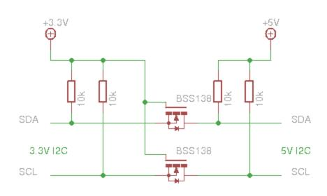
This is primarily because an I2C compliant device running from 5v requires a value of >3.5v (0.7 \* VDD)<sup>6</sup> in order to recognise a Logic 'High' level at it's I2C input.
