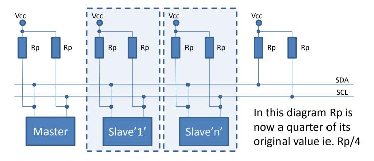
The solution is to remove some of the extra pull up resistors.
