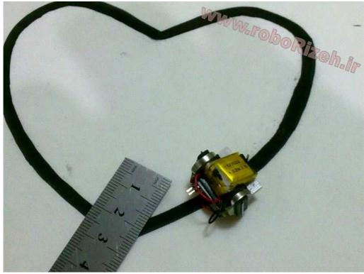
7. How to run and test: After place power connector please wait 5 second (for sensors calibration). Then place robot on course.
