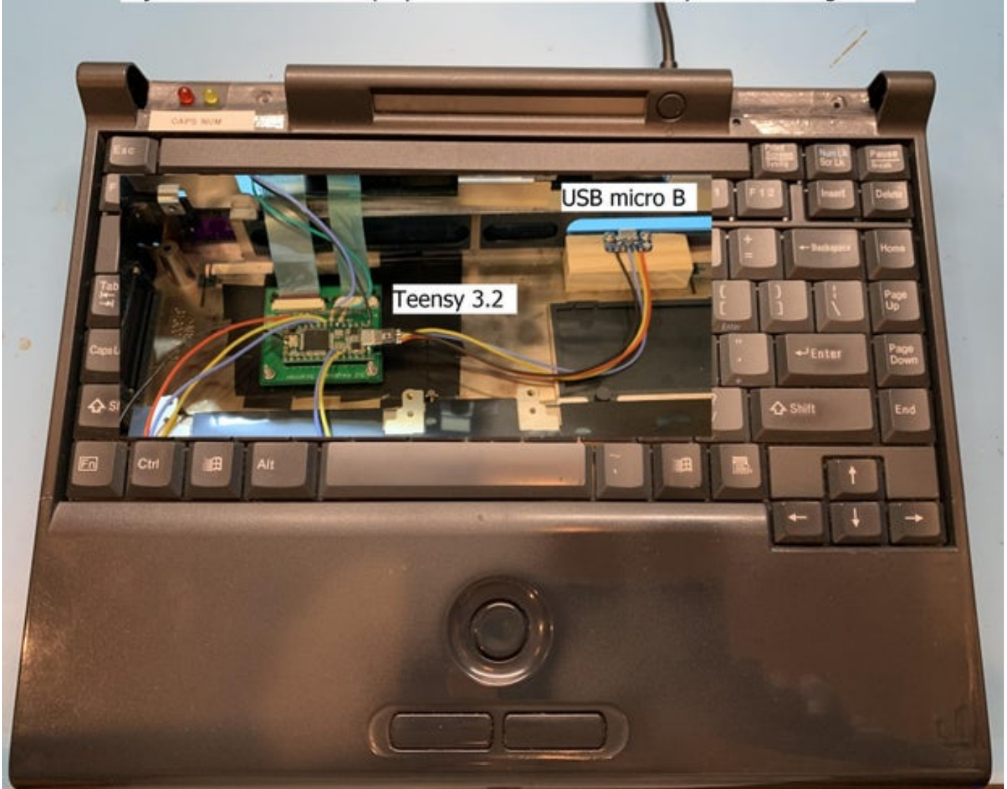
Fujitsu Lifebook 755Tx laptop base converted to USB keyboard and Ergo Trac
