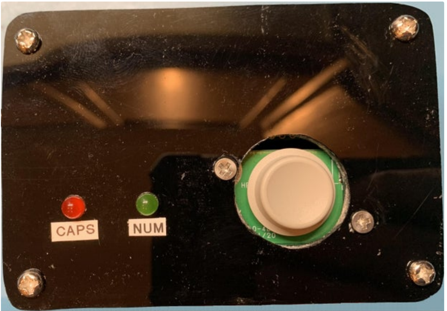
ErgoTrac pointing device mounted in a project box
