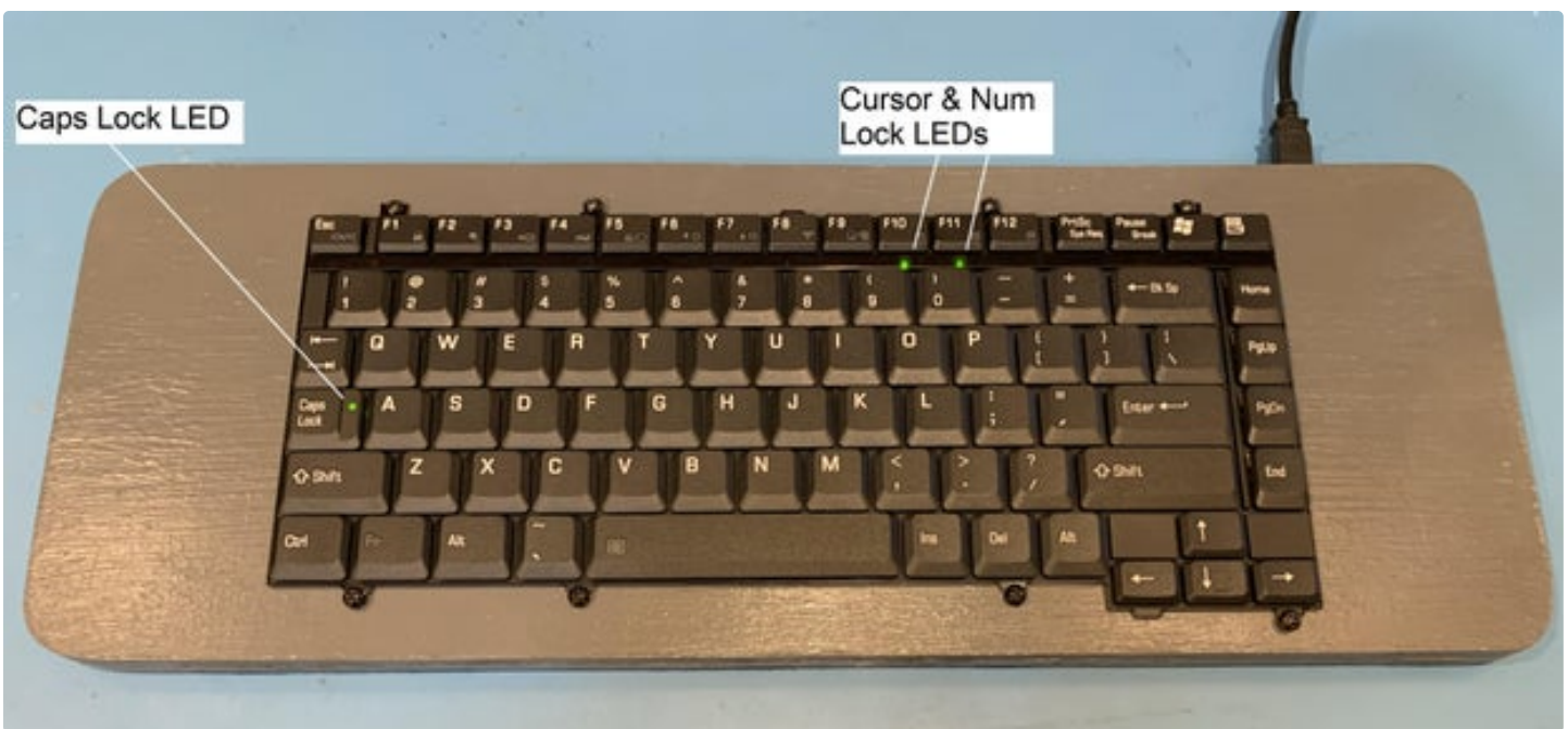
Fujitsu Lifebook 755Tx laptop base converted to USB keyboard and Ergo Trac
