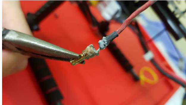
Soldering bullet head connector to the motor input wires
