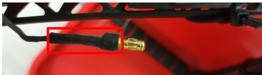
Metal connector after covered with heat-shrink insulator
