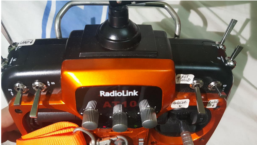
Transmitter labelled with flight modes at switches
