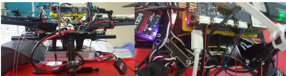
Navio2 battery connection vs cabled connection
