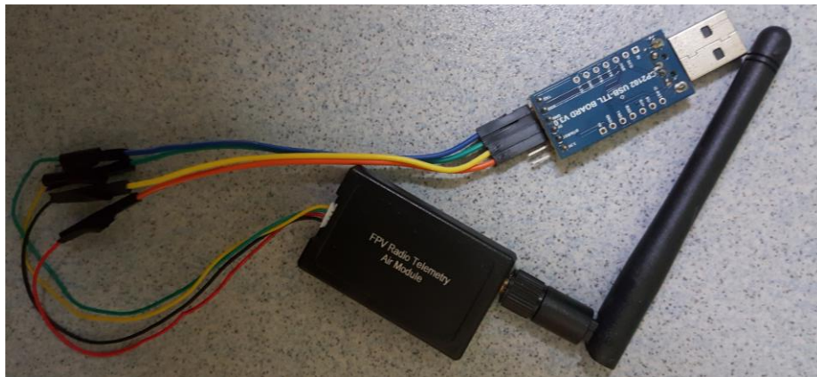
USB-TTL converter soldered to the air module
