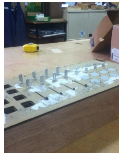
Figure 8 Testing the casing is big enough (2 Omni boards)
