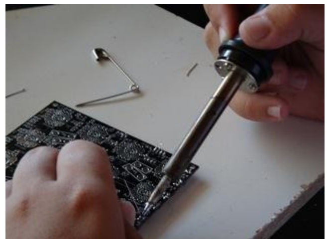
Figure 9 soldering Components into the Omni board
