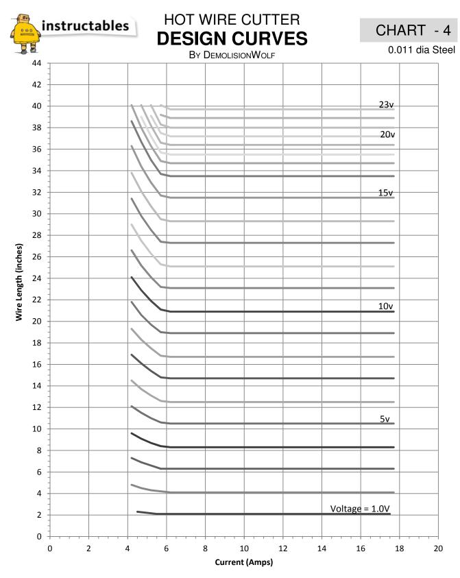
\* To increase temperature of wire during testing, decrease length by 0.5" incriments.
