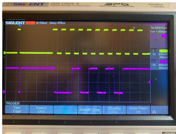
Clock and Data signals on Motorola 4824402E pins
