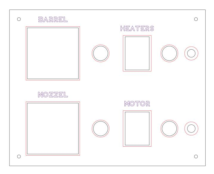
Purple - Engrave or paint/draw Red - Actual size of parts (can be ignored when cutting) Black - Holes to drill out or lines to cut
