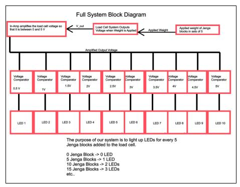
Figure 2: Full System Block Diagram.
