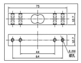
Figure 5: Mechanical drawing of load cell.
