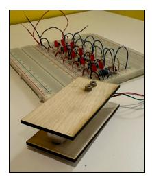
Figure 6: Image of the load cell with platforms attached.
