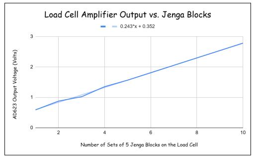
Figure 9: AD623 output voltage versus the number of Jenga blocks on the scale for a  $33\Omega$  resistor.
