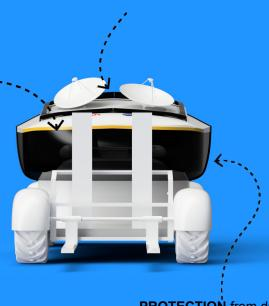
**PROTECTION** from dust and debris from the wheels.
