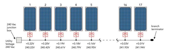
The top row of numbers is the incremental voltage rise from one microinverter to the next, and the bottom row is the cumulative line-to-line voltage overall.
