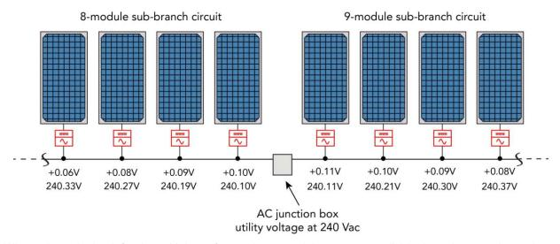
When a branch circuit feeds multiple roofs or sub-arrays, it is common to divide the sub-arrays into sub-branch circuits. It is acceptable to have different numbers of microinverters on each roof or sub-branch circuit. This is because the conductors from each Engage Cable on that branch circuit are paralleled within a junction box where all red conductors come together, all black conductors come together, etc.
