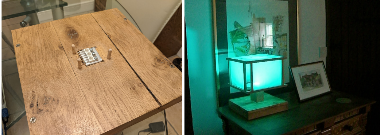
Figure 8 - The lampshade is removable, under it sits some heatsinked LEDs
