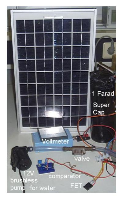
Solar pump can be used to pump water for irrigation of a greenhouse. It happens often that that the day is cloudy and the current from a solar panel drops to ca 10 % of peak, that is no longer enough to drive a motor. Solution would be to have an overdimensioned panel (100 W to drive 10 W pump).
