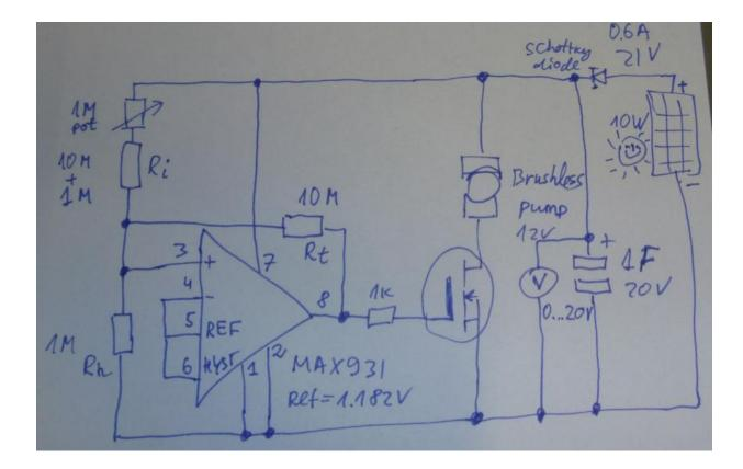
1F 20V Super Cap is from car audio (ca 25 EUR). The cap I have, is having leakage current at voltages above 13V. It might not be to run it in such mode as electrolysis will take place.
