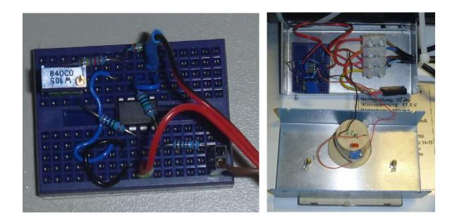
Test construction was done on a solderless breadboard and later fitted into outdoors-qualified enclosure.
