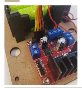
Connect the 4 wires of a male-to-male wire bundle to the 4 pins on the motor controller
