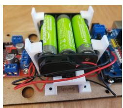
Connect the 9V battery snap to the 6AA battery holder pack
