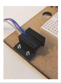
Carefully push the wires into the Bluetooth module clip until the even with the front of the clip, making sure not to cross the wires
