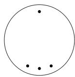
A 1.5" diameter circle with 4 1/16" drill holes about 3mm in from the edge.
