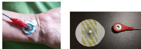
Figure 2: examples of a custom electrode clip (left) and a typical electrode clip of an off the shelf AD8232 module cable (right)
