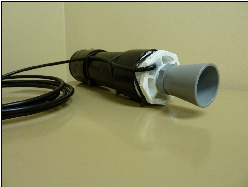
Figure 9: External antenna cable inserted through case bottom and sealed with silicon.
