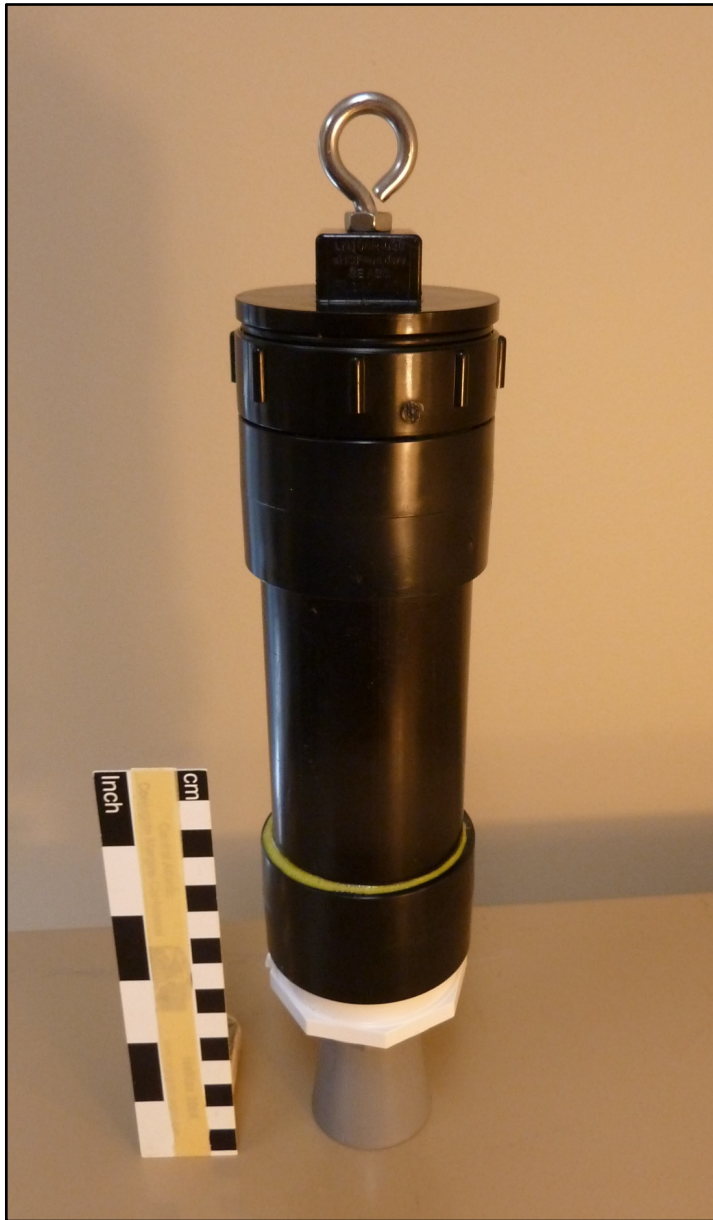
Figure 1: External view of meter. Dimensions: 320 mm long (tip to tip), 50 mm diameter. Temperature and EC sensors are not shown; they connect to the meter case with cables.
