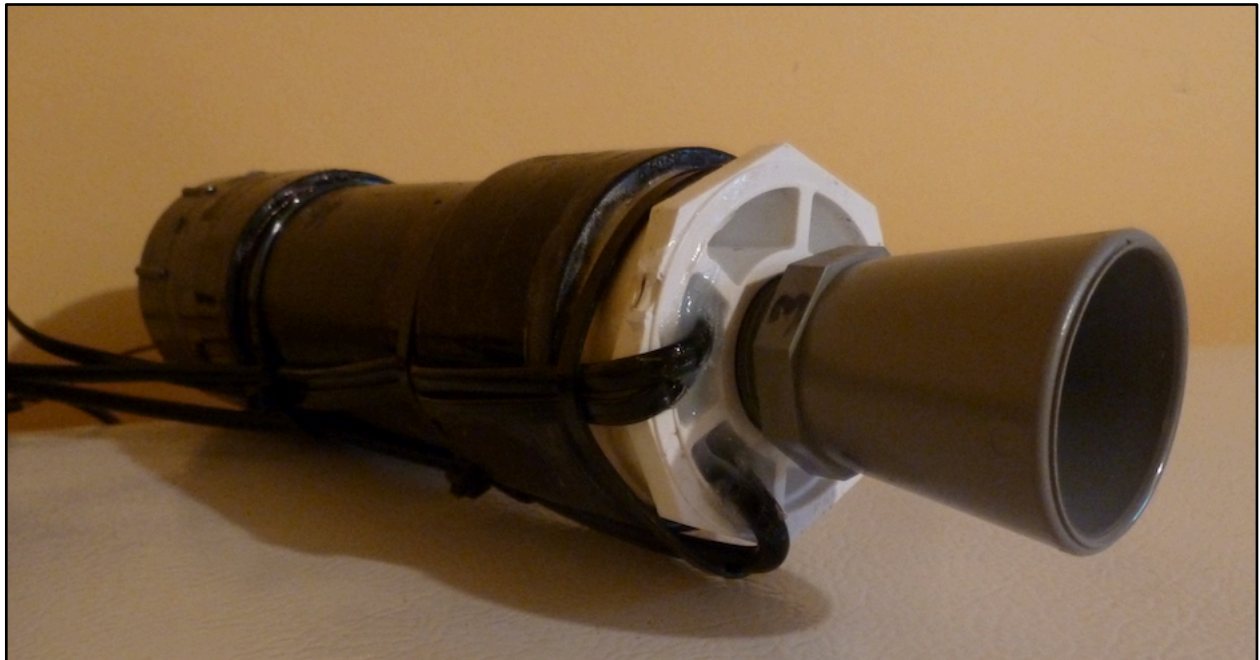
Figure 5: Sensor cables inserted through bottom of case and sealed with silicon.
