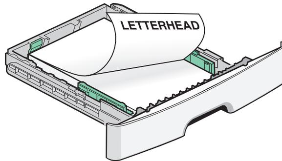
6 Squeeze the width guide tabs on the right guide, and slide the width guides to lightly touch the side of the stack.
