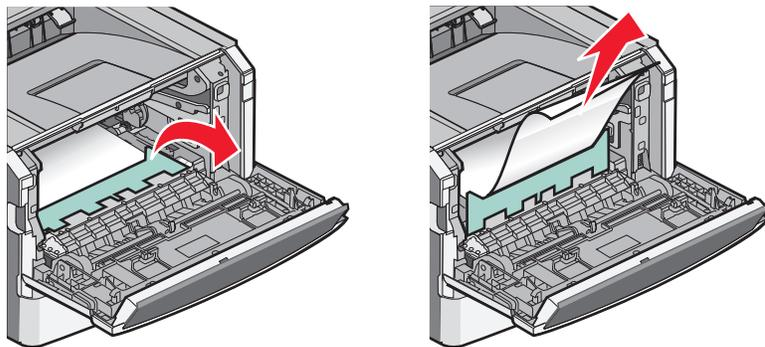
**Note:** If the paper is not easy to remove, then open the rear door to remove the paper.
