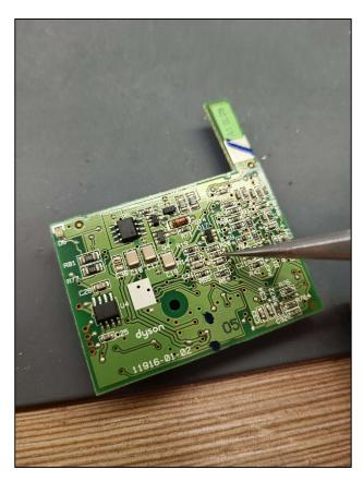
2. Thermistor (10k) must be removed from the dyson battery and connect direct to white connector or just connect 10k resistor insted of original thermistor.
