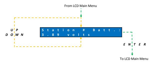
Press **UP** & **DOWN** buttons to cycle through stations Press **ENTER** button to return to the LCD Main Menu
