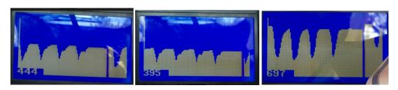
Noticed that 10 seconds keeping max revolutions gave an effect only for the first few seconds. This is probably pressure wave that pushes out the dirt. So in next tests pressed gas pedal for ca 2 seconds then let to calm down. Repeated up to 10 times. There was a trend that absorption dip became less. But 30 km was not enough.
