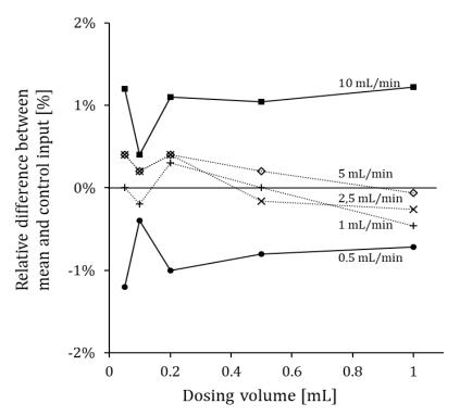
Trueness measured as difference between mean and control input over various dosing volumes and flow rates; each data point is the mean of 5 measurements
