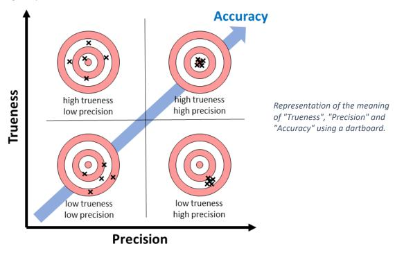
The investigation of trueness showed a dependency on the flow rate. The one-point calibration performs 30 rotations within 30 seconds, leading to a flow rate of approx. 3 ml/min with an inner tubing diameter of 0.8 mm. Close to this velocity, the trueness of the pump is +/- 0.5%. For a significantly faster or lower speed, the average value is about 1% higher or lower as the set value.
