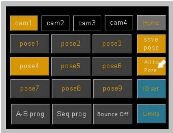
The **[All to Pose]** button is a new feature on V6.03 which offers you a quick and easy way to have all 4 camera systems move to the same Pose/Preset number. This may be very useful if for example you want all 4 of your cameras to target a particular Actor on your set quicklay for example a lead singer or the drummer etc. Using the function requires some pre- thought regarding how you set up your Poses / Presets beforehand.
