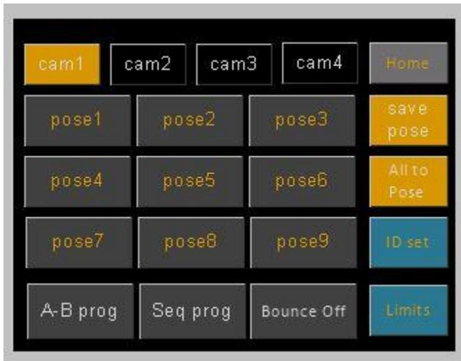
With the latest update the Digital Bird WIFI PTZ menu now allows you to set up to 4 camera systems for live camera moves. Each camera system may consist of a Pan Tilt head combined with any number of other Digital Bird Devices for example a slider or the mini Jib.
