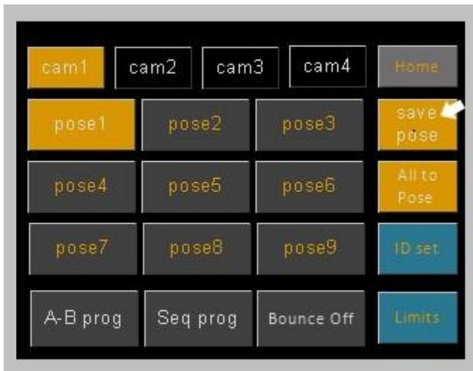
Poses or Presets are recorded positions for all axes on your system which can be recalled with the tap of a button. Poses saved using the WIFI controller can also be recalled from OBS using the VISCA connection however vMix does not use the memory slots on the head but keeps its own record of the positions and will therefore not recognise presets saved from the WIFI controller.
