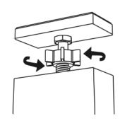
Turn the adjusting screw clockwise to tighten against the ceiling.
