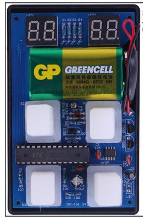
Step 21: Place 4pcs Button on LED. Just need place and no need to fix for now.
