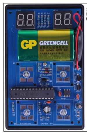
Step 20: Install 1pcs 9V 6F22 battery. Note: Users need to bring your own battery which not include in package.
