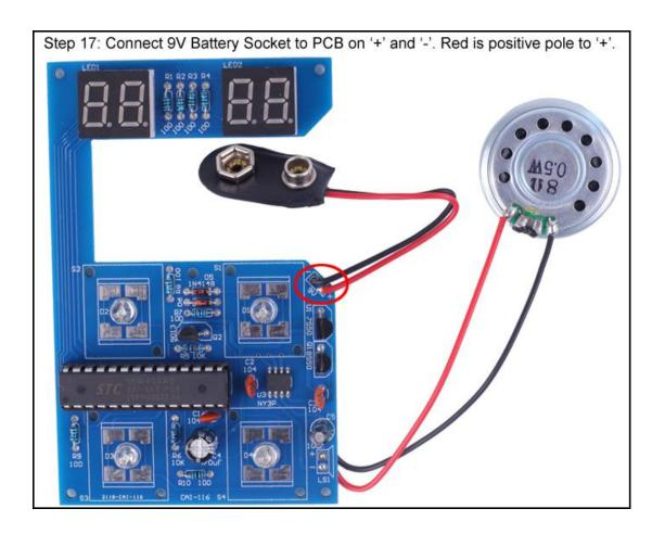
Step 18: Use a plastic bag to cover the speaker to avoid that the metal on the surface of the speaker directly touches the PCB pad, which may cause a short circuit.
