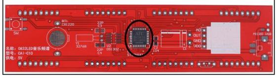
Step 4: Connect others pads on STC8H1K16 by tin and soldering iron. Note: This is just the most basic installation method if your welding tools are not complete.
