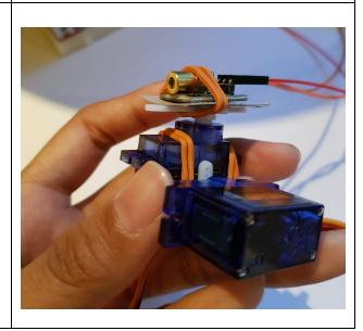
6 Put something hard under the laser module. This will allow us a larger and sturdier surface to attach the laser module to the servo. I used a scrap piece of cardboard and tape.
