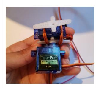
Tuck in the cable of servo 2 under the rubber band as well. This is so that when the servo rotates, the wire won't be caught in the motion.
