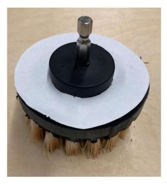
4. Use a smooth, slow, and consistent rotating motion to cut out the rest of the bristle attachment, following the outer edge of the guide.
