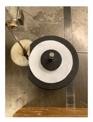
3. Set up the bristle attachment set up in the bandsaw with the hex bit facing up. Make a straight cut tangent to the outer edge of the guide.
