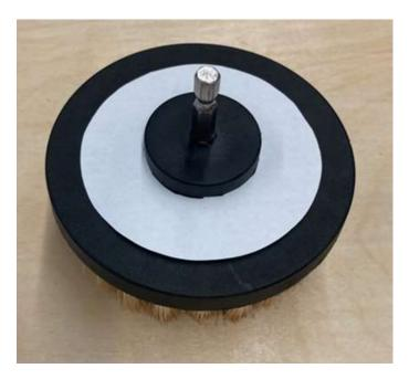
2. Place the cut guide on the top side of the 4" bristle attachment. If it doesn't fit snug, you can use tape to secure it.
