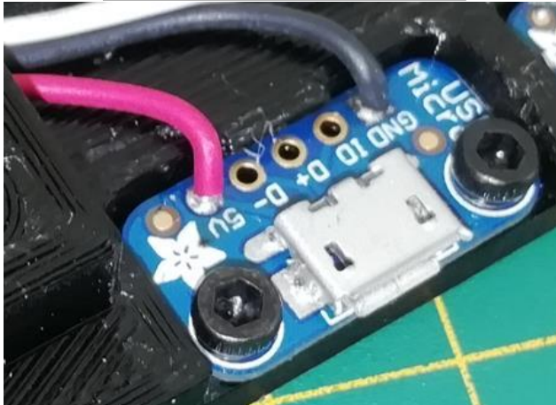
microUSB breakout board: Wire soldering orientation
