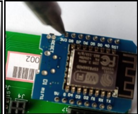
Step 3. Apply just enough solder to cover the pin hole.
