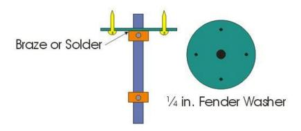
Insert the longer part of the shaft from the top side of the Top Plate, thru bushing both bushings.
