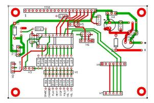
7. Install the Radial Capacitors; there are two of them, C1 and C4.
