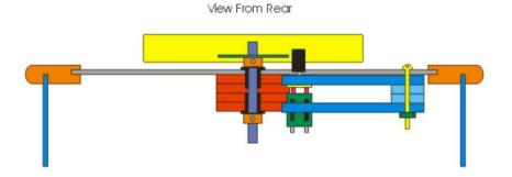
Install the Spring from the Motor Mount to the bolt/screw hole as shown in the CAD drawing.
