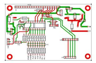
6. Install the Headers; these are used to make connections to items off the PCB such as
