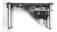
If you are connecting the TCS230-DB to the motherboard via the extension cable (p/n 800-28301), attach the spacers directly to the TCS230-DB using the unused short screws provided with the motherboard.
